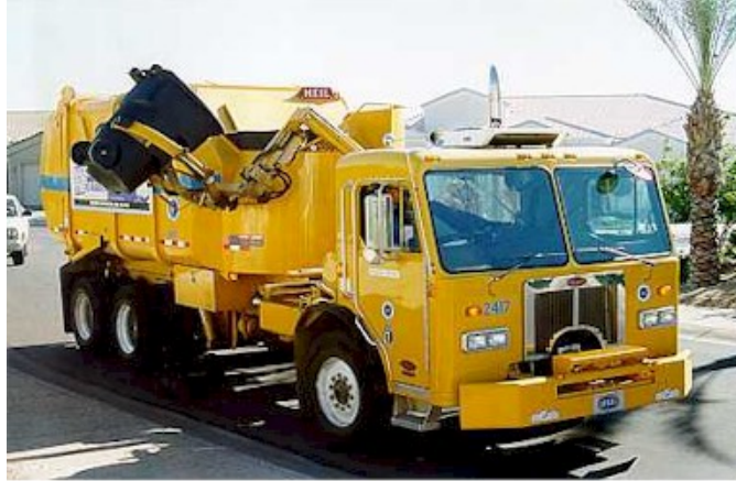
Exhibit 20. Modern Application of Automated Side-Loaders By the City of Scottsdale, Arizona
